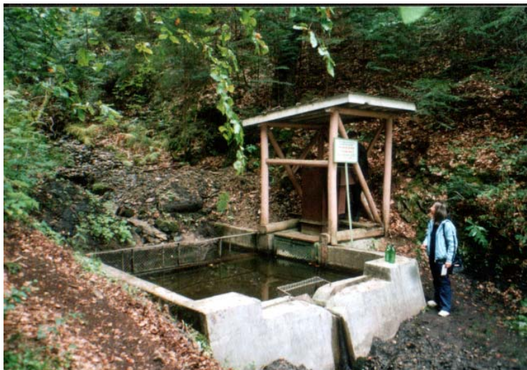
Fig. 4: Accumulation tank for bed sediments at the Yundola experimental site in Bulgaria.
