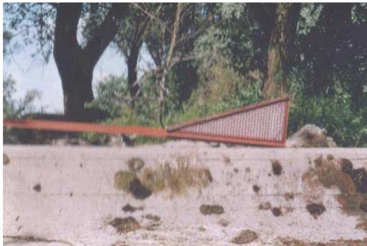
Fig. 5: Steel frame and nylon mesh to catch bed sediment load on the crest of the spillway at the Orizare open stage pit for abstraction of sand and gravel in Bulgaria.
